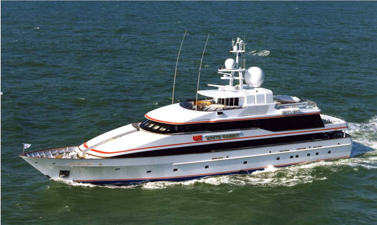
The original White Rabbit carried an impressive array of toys, but was significantly reconfigured during the refit. A 1.75m section of her stern was cut off and a new 5.25m stern section was added, extending the LOA by nearly three metres. More impressive, though, is the resulting increase in deck space with all decks being extended. Pegasus now features 265 square metres of outdoor entertaining areas
